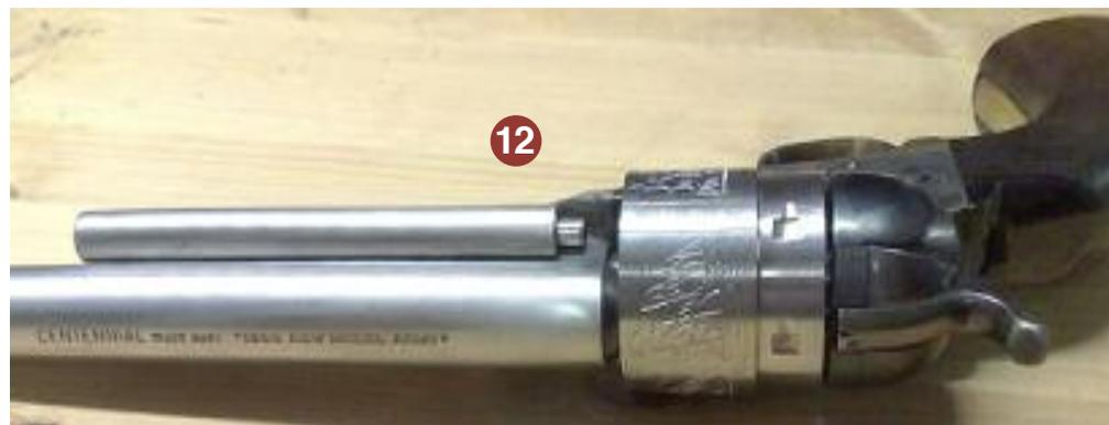
MODEL ARMY" has been maintained. (Photo 12) She is now ready for the master's finishing touches: Installation of the .429 diameter liner for my .44 Colt inside lubricated bullets, adjustment of the sights to hit POA and finally, the rust bluing of the barrel assembly, new cylinder, and other
