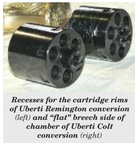
*Recesses for the cartridge rims of Uberti Remington conversion (left) and "flat" breech side of chamber of Uberti Colt conversion (right)*
