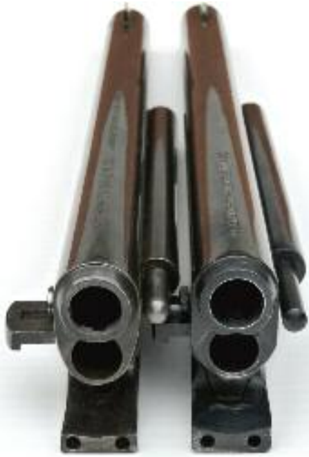
Comparative barrel view— Centaure R1 (left) and Uberti RII (right)
