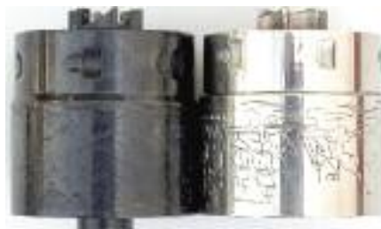
Top view of same conversion cylinders. Note gas ring of Uberti (left) compared to period correct Centaure without one (right)
