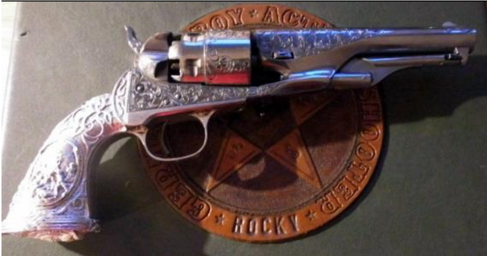
Marshal #12677: Navy sized tiffany grip requires cutting the front strap of the triggerguard to size
