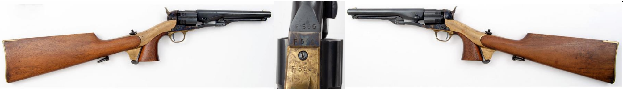
Impressions of Cavalry #F566: MADE IN BELGIUM stamped on left side of yoke, #F566 on barrel lug, frame and trigger guard
