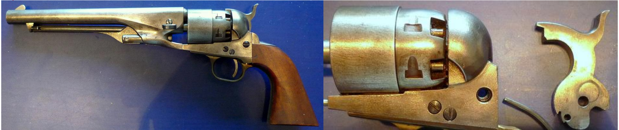
RNMA #7: steel seems to lack the finishing, no logo, no proof marks is present
