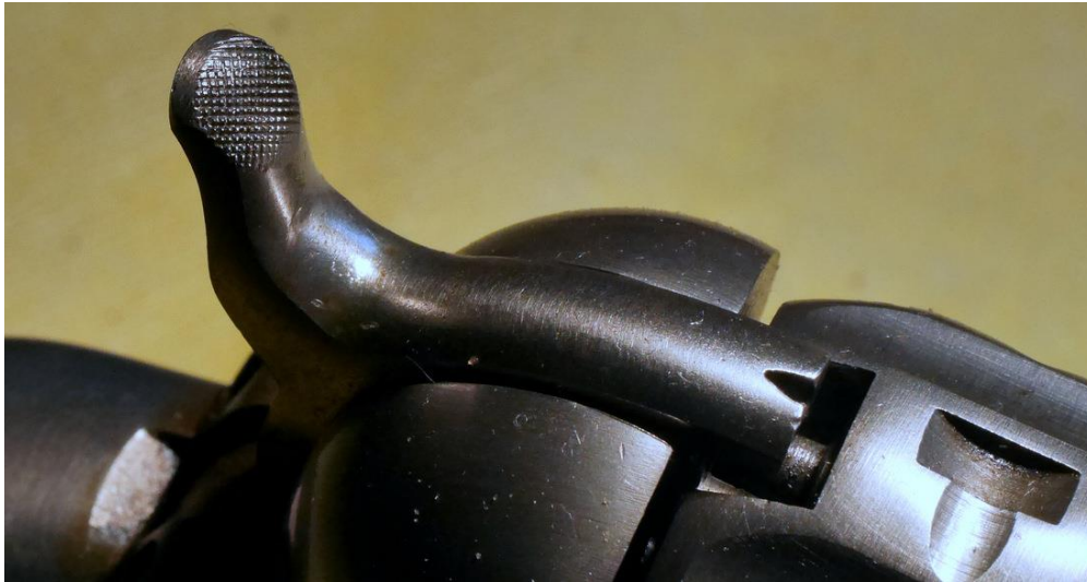
From left: regular crosshatch pattern of hammer spur serrations vs. #13988's straight groove pattern
