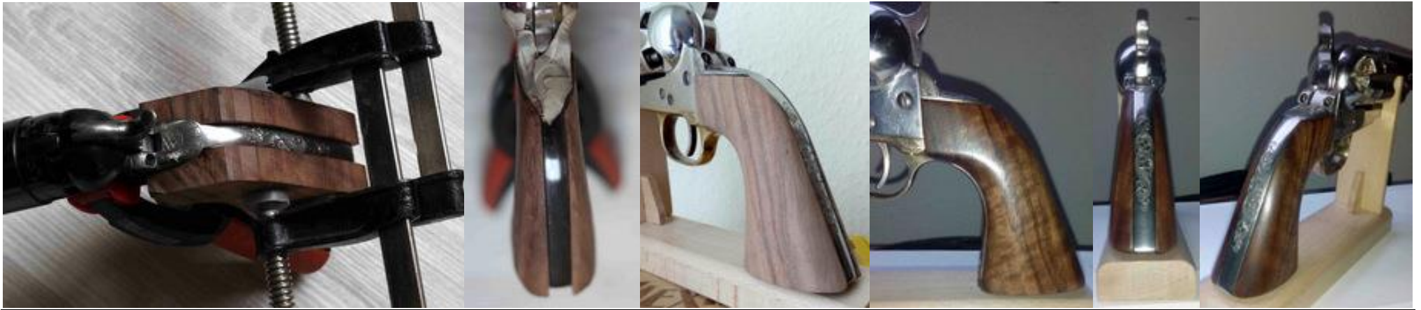
Making and fitting the new grip for #13988
