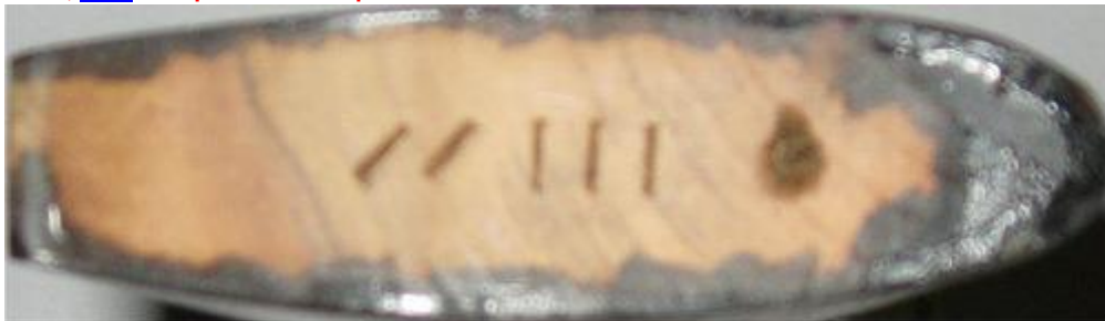
FAUL shoulder stock #F11166 from 1971: assembly nr. 23 stamped on butt plate and hacked into wood
