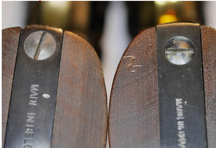
From left: 2 nd version or beefy vs. 1 st version or small butt screws
